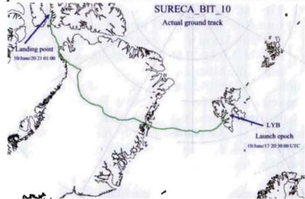
Figure 4. Trajectory prediction performed four hours before landing
