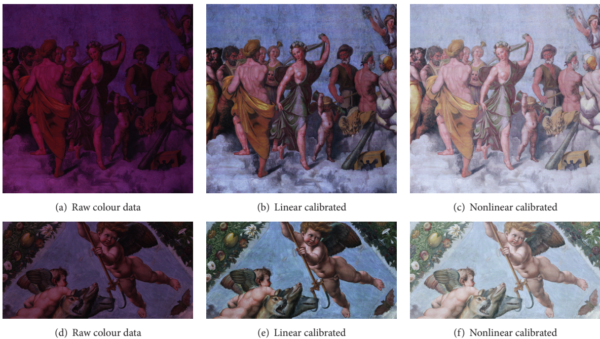
FIGURE 12: RGB-ITR raw data and linear and nonlinear calibrated colour textures of real scene at 7-9 meters of distance.
