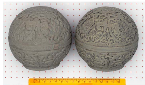
Figure 18: The colour-enhancing technique: a comparison between the plain replica (left) and the version with colour enhancement (right).
