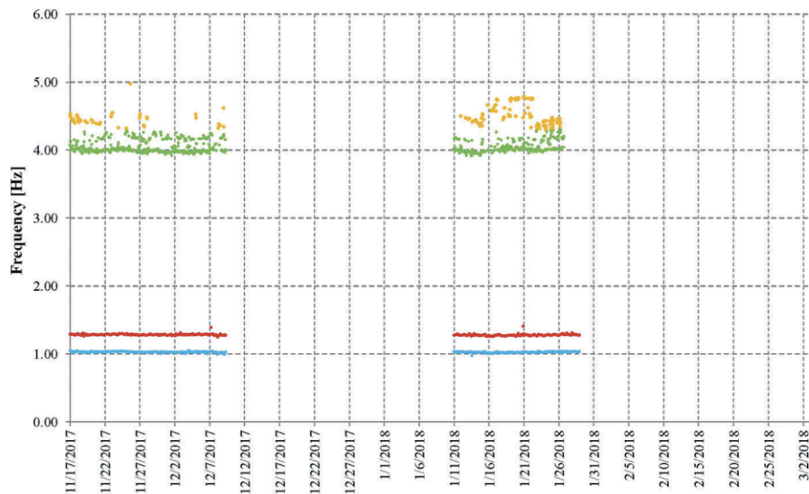
Figure 8. The tower's first four natural frequencies [Hz] detected by SS20 velocimeters during the monitoring period.
