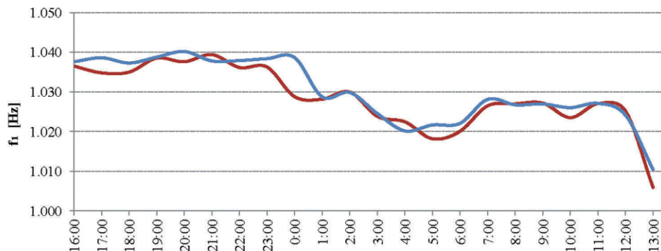
Figure 10. The tower's fundamental frequency obtained via AGI stations (blue) and SS20 stations (red) data from 7 to 8 December 2017.
