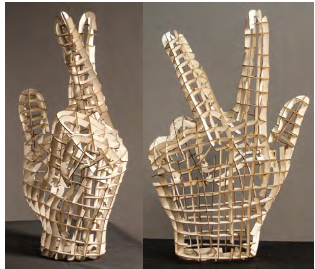
Fig. 17: Our algorithm applied the ‘hand’ model. The arrangement is composed of 122 pieces.
