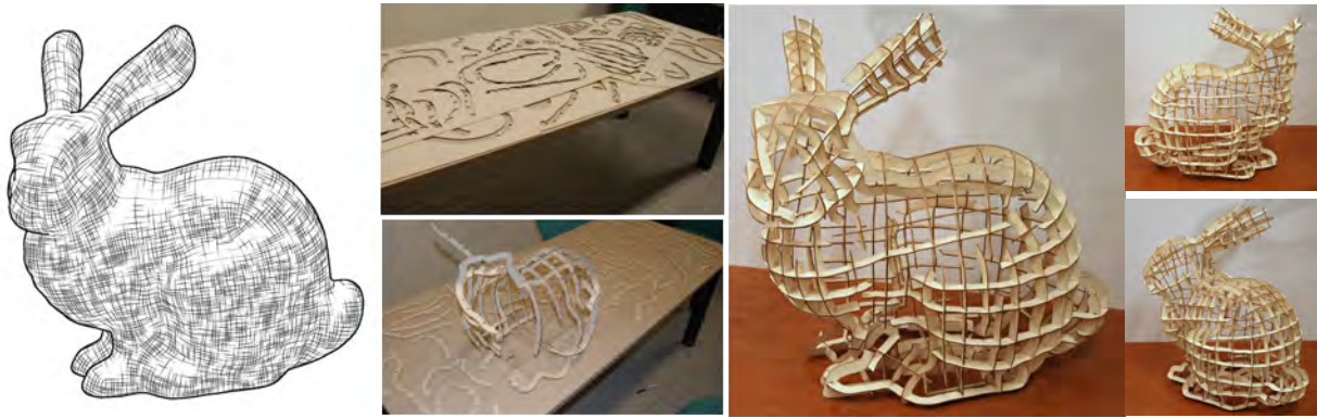
Fig. 1: Given a 3D shape with a smooth cross-field, we generate a set of planar slices that can be interlocked in a self supporting structure.
