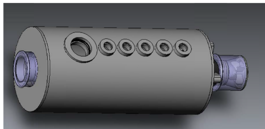
Figure 1.12: A detail of the store chamber's design
