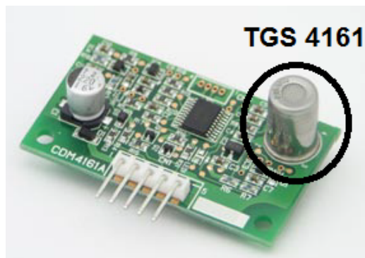
Figure 2.20: AM-4-4161 module for carbon dioxide sensor TGS 4161. The sensor is placed on this special microprocessor, which allows an accurate reading of carbon dioxide concentrations.
