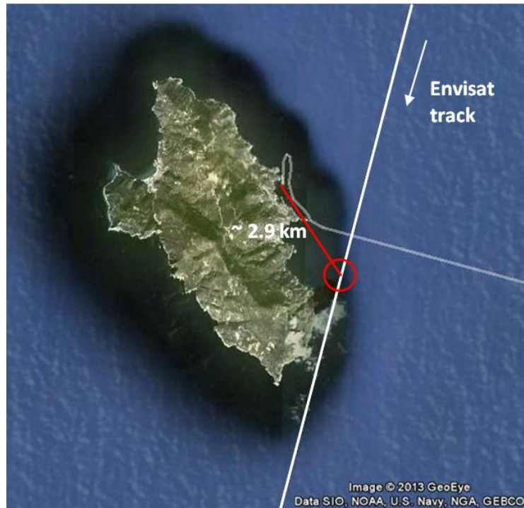
Fig. 4: Concordia ship route (grey), RA-2 Envisat orbit for cycle 111 (white) and position of the apparent target (red circle). The red line connects the apparent target with the final position of the ship (image from Google maps).
