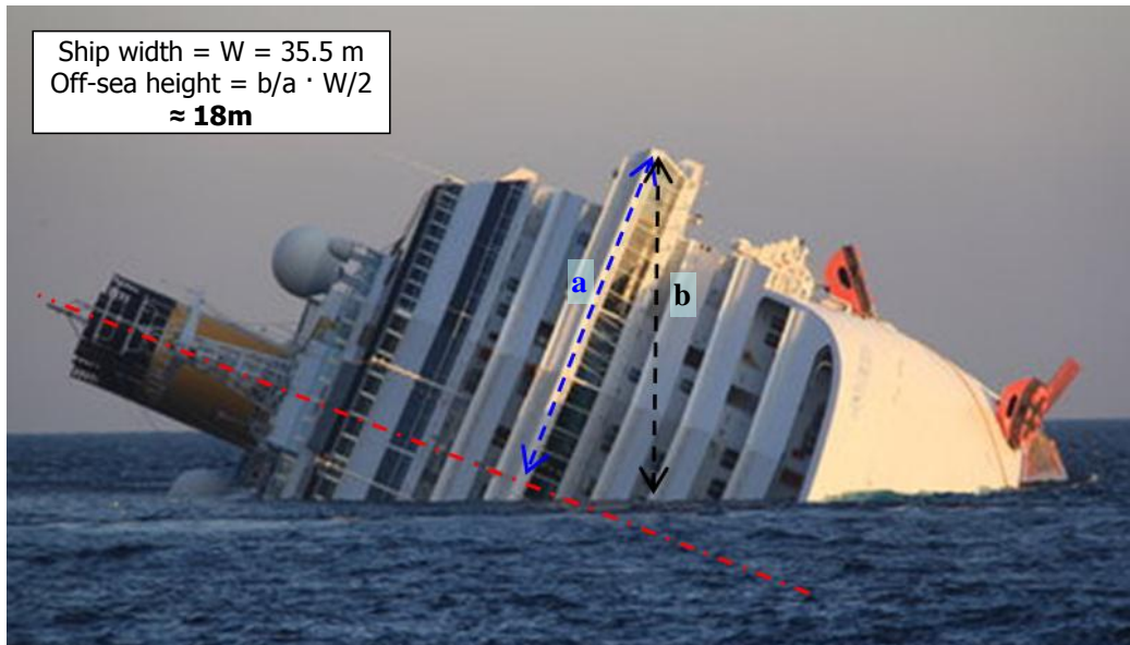
Fig. 6: Calculation of the off-sea height of the Concordia ship, based on the proportions between known dimensions.
