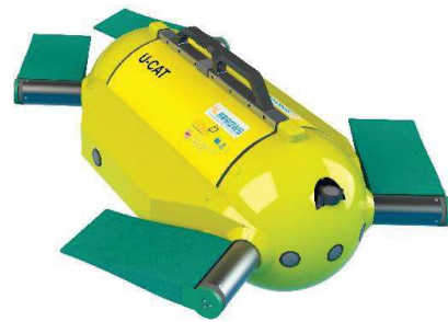
Fig. 5. The biomimetic AUV U-CAT
