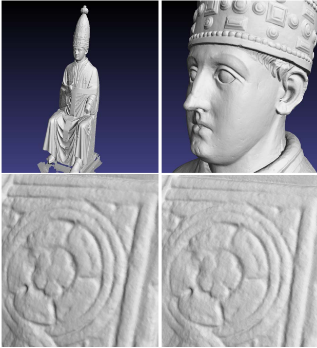
Figure 8: Big statue rendered in a browser: original PLY file, 84M triangles, 1.6GB; uncompressed model, 2.54 Gb; compressed model, 158 Mb. Top left: the full compressed model, top right: a detail. Bottom left: a detail of the uncompressed model. Bottom right: the same detail of the compressed model
