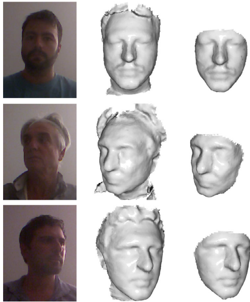
Fig. 9. 3D geometric reconstruction results. RGB image (left), 3D reconstruction for morphological analysis of cardio-metabolic risk (centre), and personalised mask for face tracking (right).
