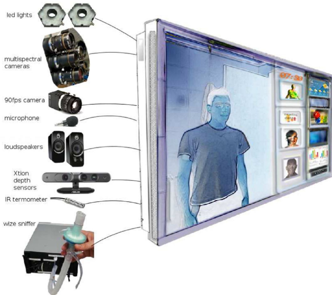
Fig. 1. Illustrative representation of the Wise Mirror. On the right widgets panel with the user graphical interface, optionally this may also include: clock, weather forecast, news, etc. On the left pictorial representation of different devices used for data acquisition.
