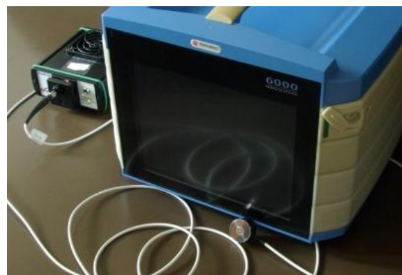
Figure 11. Fiberoptic probe with local heater for measuring skin microcirculation response Perimed AB, Järfälla, SWEDEN [[4]].
