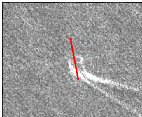
Figure 9. Azimuth line direction. The wake search is performed on the red linear subset. (COSMO-SkyMed Product—© ASI 2016 processed under license from ASI—Agenzia Spaziale Italiana, all rights reserved, distributed by e-GEOS).
