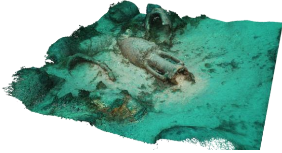
Fig. 4. 3D reconstruction of an amphora wreck by means of a Structure from Motion based procedure.
