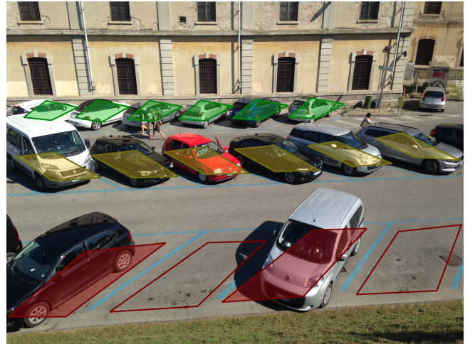
Figure 4: Sample of the interface with a view from a smart camera and the visualization of available and occupied parking spaces.
