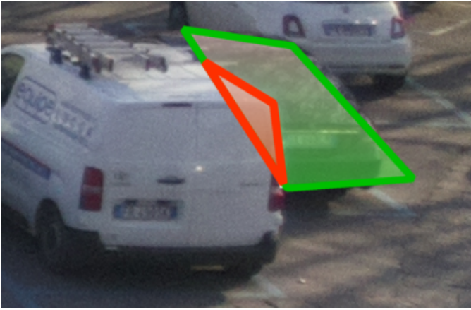
Fig. 5. Detail showing the overlapping and occlusion of a parking space with the portion belonging to the actual occupying vehicle.
