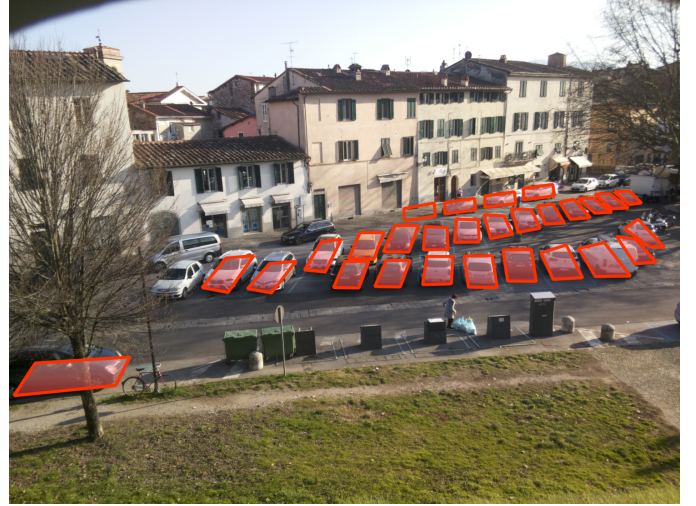
Fig. 4. Sample of the interface with a view from a smart camera and the visualization of available and occupied parking spaces.
