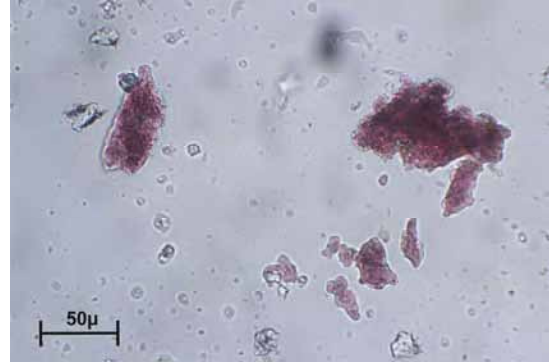
Figure 6: Micro-photo of the crushed-grains of the micro-sample no. 126372-F in reflected light and parallel nicols (PPL), 25x lens and 50 length scale, which shows elements that appear transparent and an overall pinkish colour with fine dots ranging from bright red to brown within them (Photo: C. Gratziu, A. Moscato).
