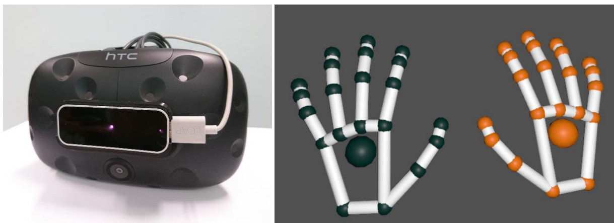
Figure 2: (Left) Leap Motion device mounted in front of the headset of the HTC Vive. (Right) Stylized model of the hands tracked by the Leap Motion.
