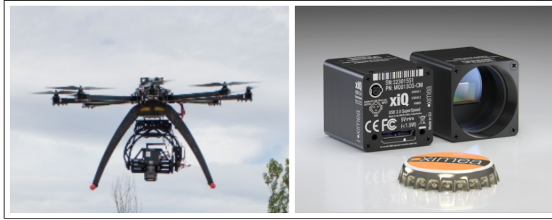
Fig. 1. The ISTI-CNR drone used for this research (left) and the Ximea XiQ high speed camera used to run SLAM algorithms on the NVIDIA TX1 processor (right)
