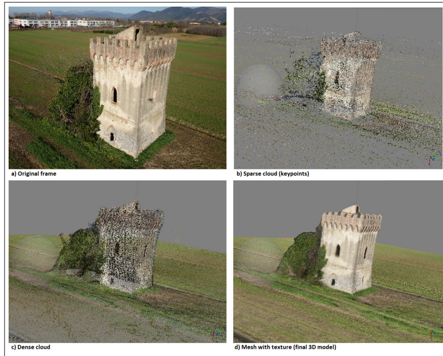
Fig. 3. a) the original aerial view from the drone; b) the first step of the algorithm selects reliable key-points; c) the dense point cloud is computed; d) the final 3D model is a polygonal mesh with texture from the original frame
