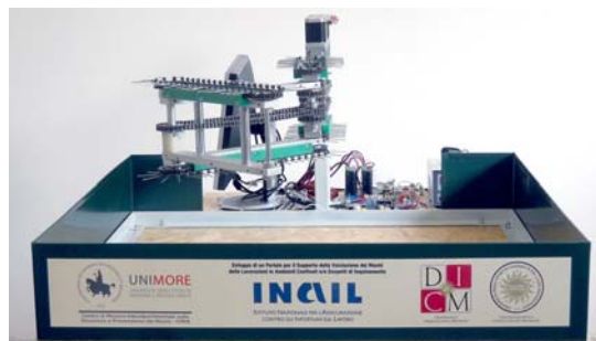
Fig. 1 - Robotic arm prototype to remove skins by wine fermentation tanks.
