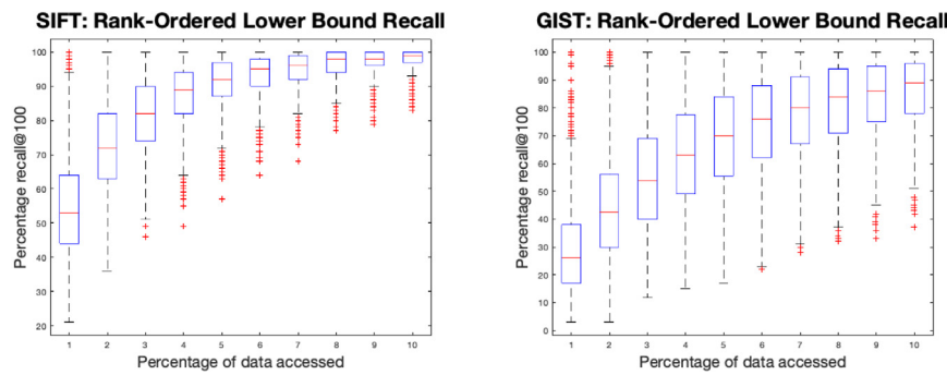
Fig. 9. Ranked order results for SIFT and GIST collections of 1M data objects. For each of 1000 queries, the four-point lower bound is used as a filter to find a fixed-size set of promising candidates, which are then checked within the original space. The X-axis gives the percentage of the 1M data which is accessed, the Y-axis shows a boxplot of the percentage recall, for a 100 nearest-neighbour ground truth, across all queries.
