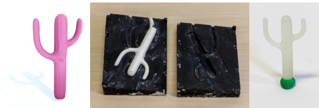
Fig. 10. For a simple object, our method can derive a single two-piece rigid mold as in [Stein et al. 2019].
