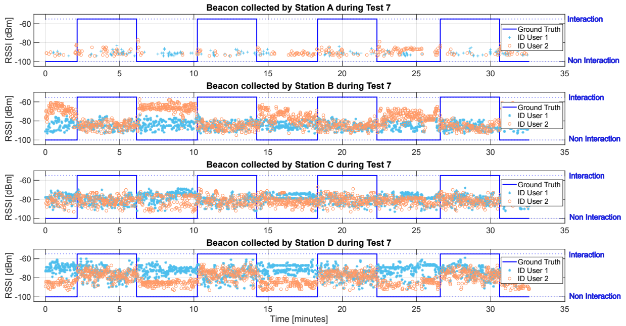
Fig. 4. RSSI variations of beacons recorded from 4 stations at different distances from the same interaction point during the Interaction and Non Interaction stages.
