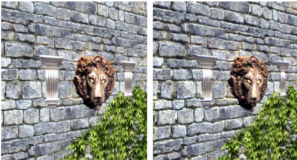
Figure 2.19: Rendering with Parallax Mapping. Left: A flat wall rendered with standard texture mapping. Right: the application of parallax mapping modify texture coordinates in a view-dependent manner, resulting in an illusion of depth which produces a parallax effect whenever the relative position and orientation of the scene and the observer change.
