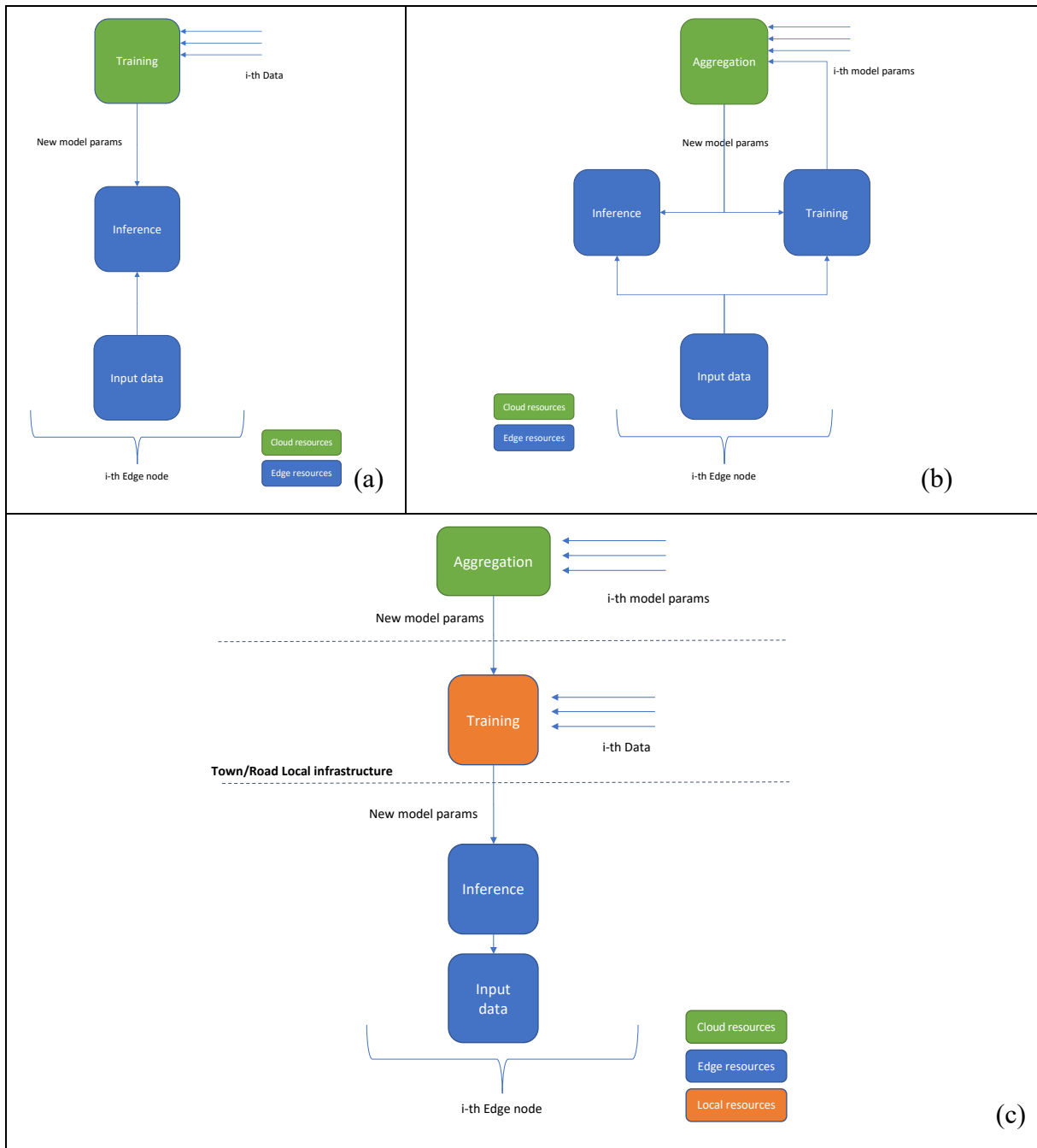
Figure 4: Centralized Learning (a), Federated learning/ Training at the edge (b), Hybrid (c)
