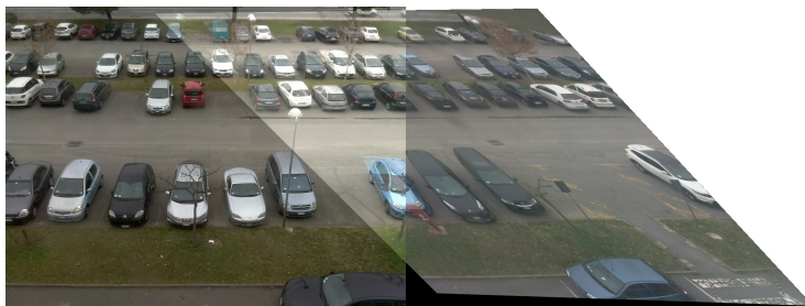
Figure 3: Example of concatenation of two images using a homographic transformation, where it is also visible the overlapping area between them.
