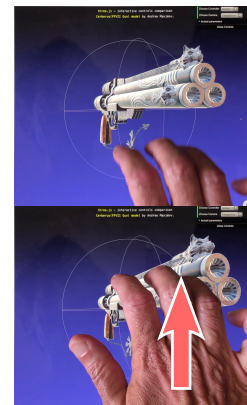
Figure 9: Field of view manipulation using three fingers.
