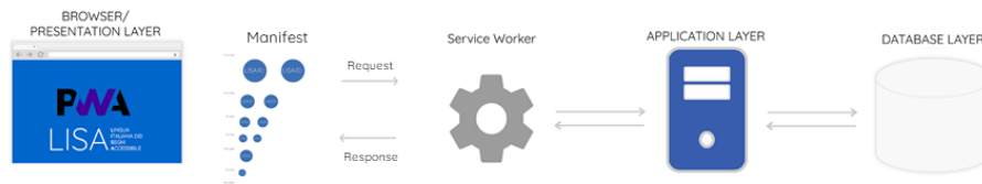
Fig. 4 . LISA Architecture showing the interconnections between the five tiers
