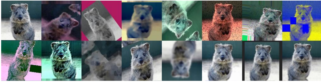
Figure 2.4: The original image (top-left) with a set of strong augmentations, altering both image geometry and pixel values. From https://github.com/aleju/imgaug .
