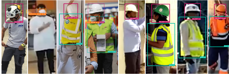
Figure 9: Examples of predictions of the PPE Detection module on our CrowdVisorPPE test set. PPE classes are color coded ( helmet , high-visibility vest , face mask ), and the detection score is reported in parenthesis.
