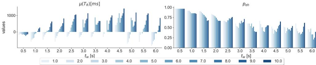
Fig. 8. Impact of the hysteresis values ( $h$  from 1 dBm to 10 dBm) to  $T_R$  and  $p_{eh}$  metrics for Algorithm A3.
