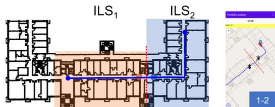
Fig. 4. Graphical representation of testing environment with two ILSs, the transition line is reported as red-dotted line.
