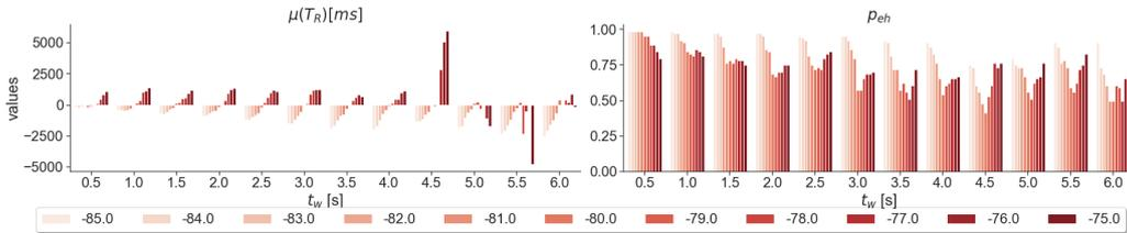
Fig. 7. Impact of the threshold values ( $\tau$  from -85 dBm to -75 dBm) to  $T_R$  and  $p_{eh}$  for Algorithm A1.
