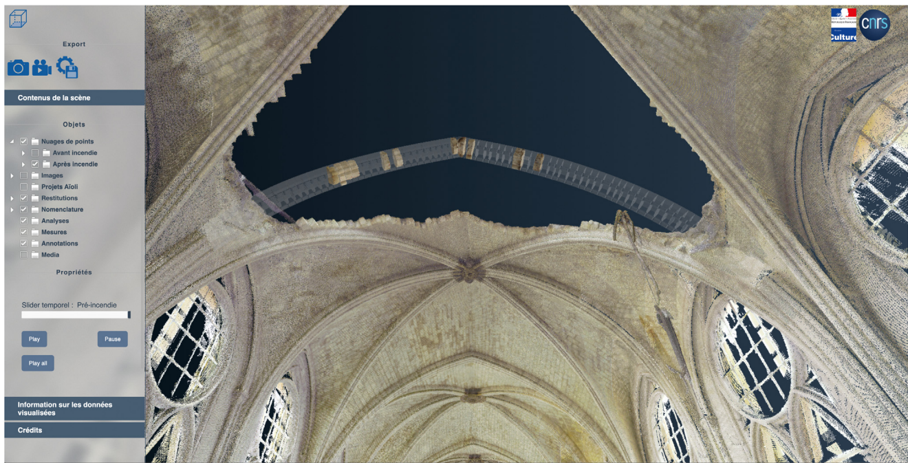
Fig. 6. Virtual anastylosis of the voussoirs of the collapsed arch in the nave of the cathedral, displayed in the NDP 3D Viewer.
