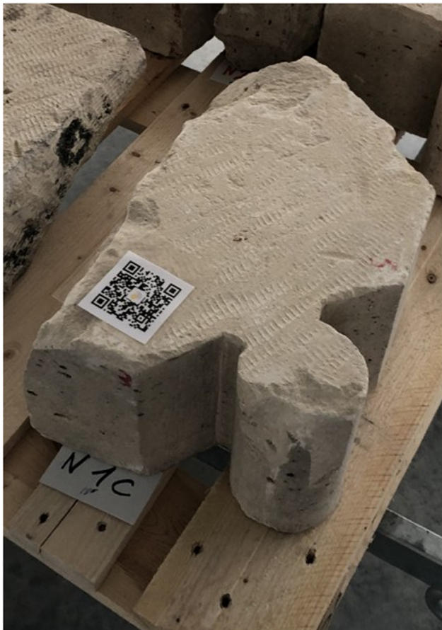
Fig. 3. QR Code of a voussoir and its digital passport in the ArcheoGRID database.
