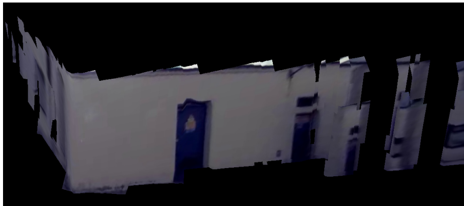
Fig. 10: A snapshot of the application with the same geometry as in Figure 7 after the fine registration step.
