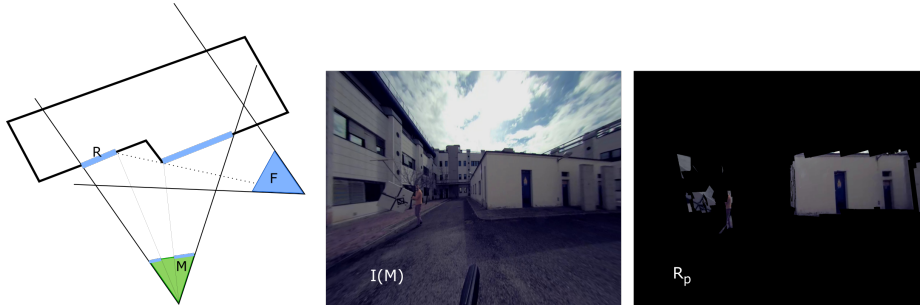
Fig. 8: The scheme shows the reference camera F and the camera to be fine-aligned ( M ). The images are the actual feed from the physical camera and the rendering with the current extrinsic parameters.
