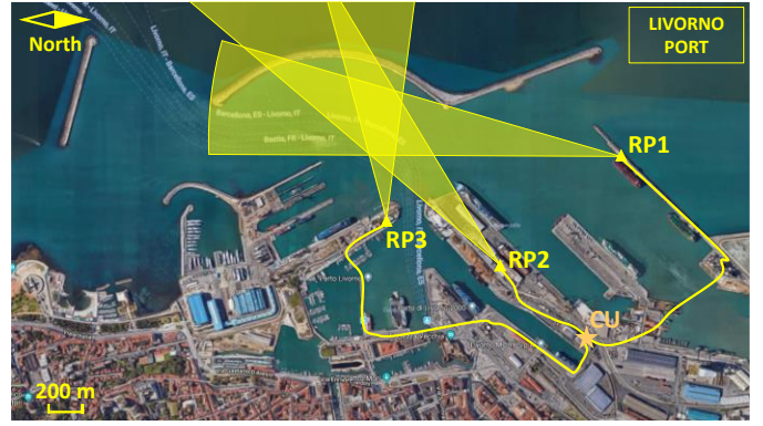
Fig. 2. Topology of the MIMO radar network in a real port for traffic monitoring. The system central unit (CU) is connected to the radar peripherals (RPs) with optical fiber (represented by yellow lines). The yellow-shadowed areas schematically depict the transmission pattern of the employed antennas.
