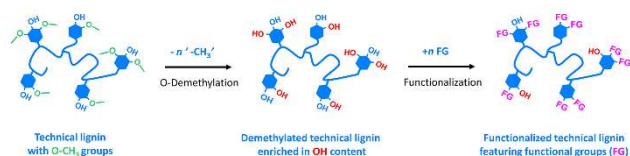
Scheme 11. Graphical representation of ODM and functionalization in the valorization of technical lignin.
