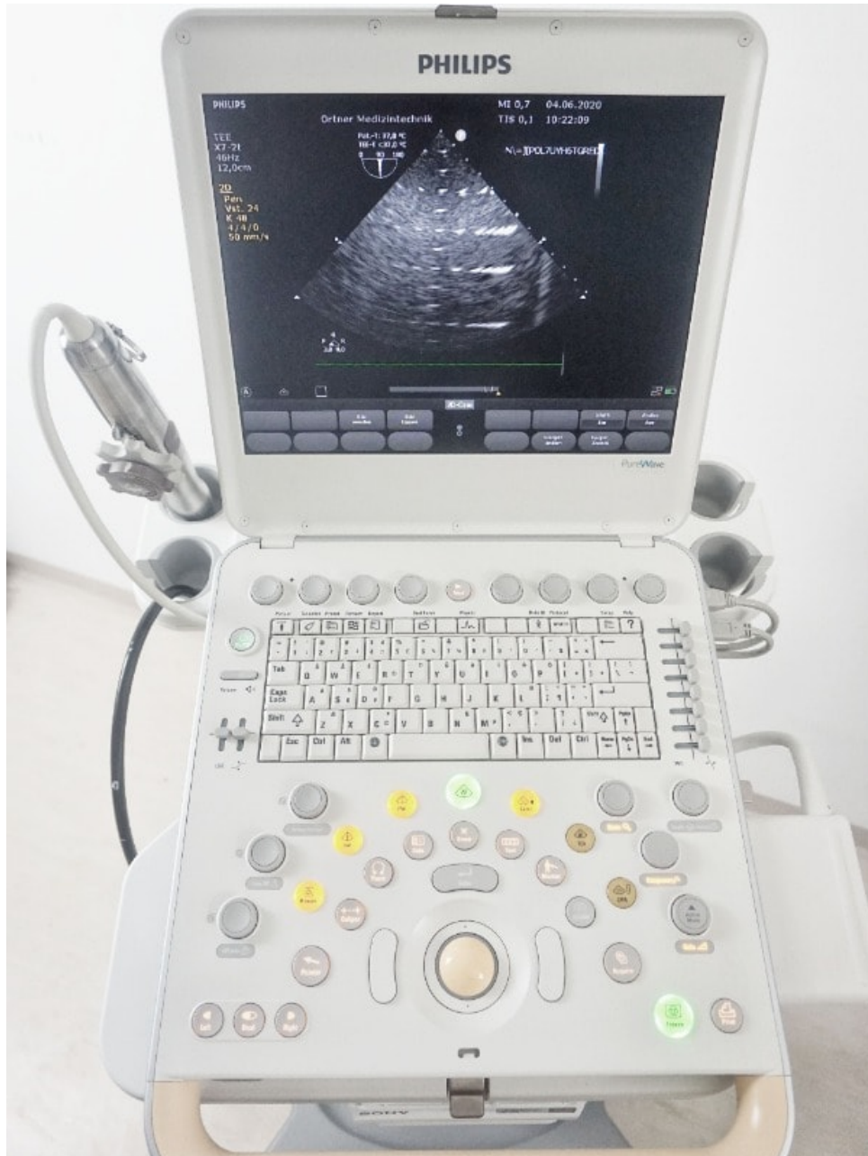
Figure 3.2: A modern example of an ultrasound device, its structure resembles that of a modern notebook, each key in the keyboard represents a setting, like Gain, Depth, etc.
