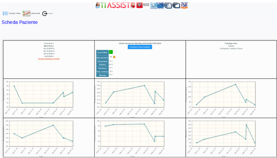
Figure 2.3: The figure portrays the Italian TiAssisto website, in which the involved physicians can monitor vitals, images, and notes from the related subjects; the system automatically detects anomalies and visually alerts the physicians.
