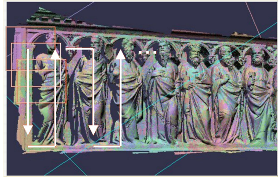
Fig. 1. Range maps are taken in a row-wise order: an example of circular stripe around a statue’s head (left); an example of raster-scan scanning order adopted for the acquisition of a bas-relief (right).
