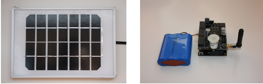
Fig. 1: Our solar energy harvesting system: The solar module KL-SUN3W (on the left) and the Waspote platform (on the right).
