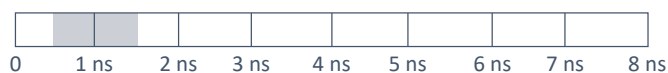
Fig. 2 Schematic illustration of the running average procedure, for an interval of 8 ns. At every 1 ns time step, the structure is obtained from the running average of all the frames included in the shaded time window, as shown only for the first step.
