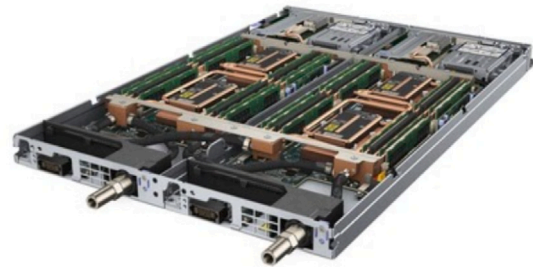
Fig. 4. Schematic of the two-phase cooling system (left) and its embedding in a server (right).
