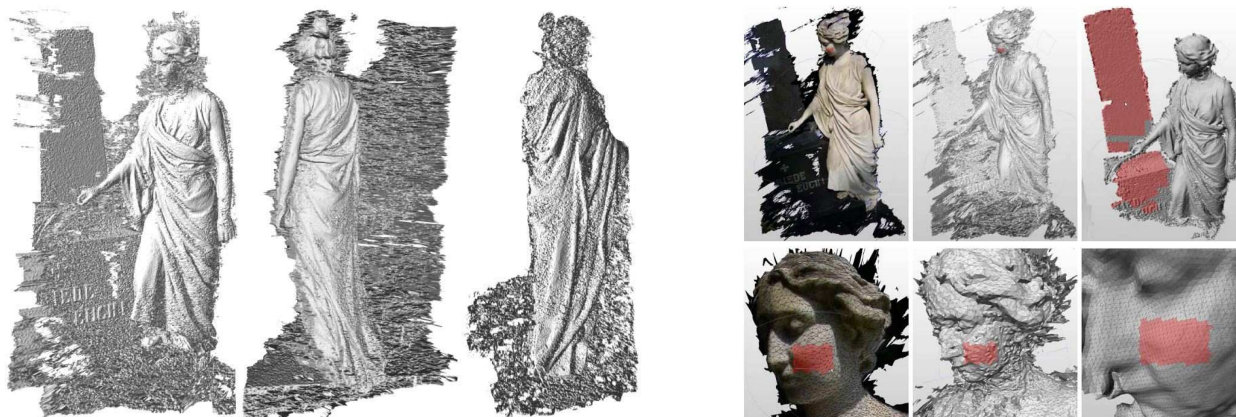
Figure 1: Creation and markup of a 3D model from range-map input. Left: Original input data, 3 out of 20 range maps taken from a statue are shown un-textured. Top right: Simplified versions of the range maps, textured and un-textured. The gravestone and the statue’s cheek were manually segmented for semantic markup. Bottom right: Several range maps were integrated and smoothed.
