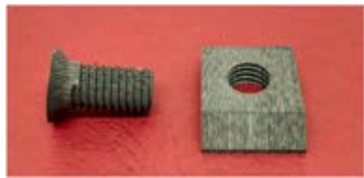
Fig. 7. Example of a screw and a nut machined by a sintered UHTCMC item produced by our group as concrete examples of components with complex geometry.
