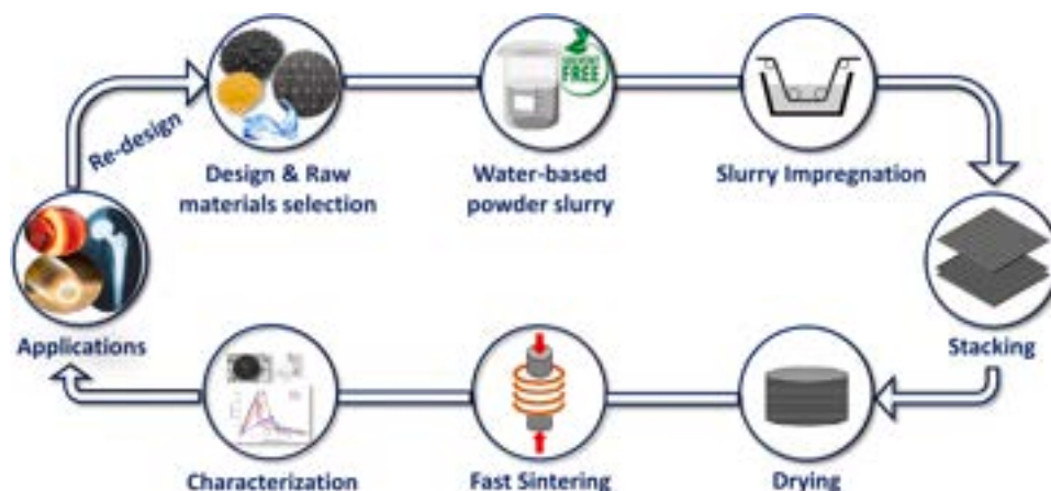
Fig. 1. Sketch of the water-based slurry impregnation and sintering process for manufacturing of UHTCMCs.
