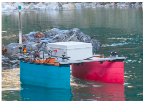
Fig. 1. The battery powered SWAMP vehicle.
