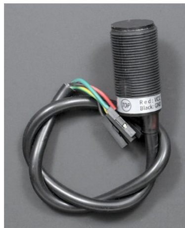
Figure 4. The IR positioning camera (courtesy of www.dfrobot.com/product-1088.html , accessed on 27 November 2020).
