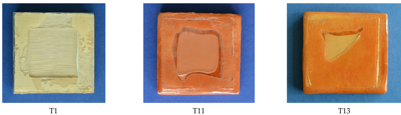
Figure 11. Tile models with artificial delamination.
