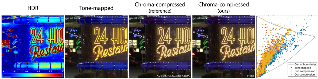
Fig. 1. Accurate and efficient chroma compression is important for the reproduction of HDR images on standard displays with limited computational resources. This study proposes a deep learning-based method for chroma compression that is up to three orders of magnitude faster than the conventional approach, while generating pixel values that similarly fall within the target display's gamut (here sRGB ). The scatter plot shows the chroma values ( x axis) of pixels within a hue slice ( h = 60^\circ ) against their lightness values ( y axis). Tone mapping cannot compress all pixels within the gamut boundaries, a problem that chroma compression is able to solve. HDR, High Dynamic Range.
