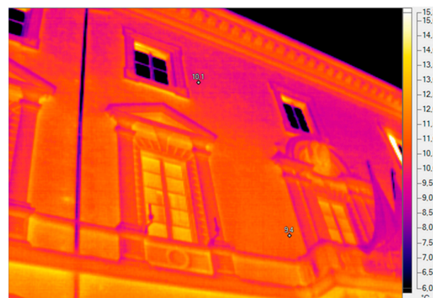
Figure 17. Marker at the measuring points of the heat flow meter of rooms 105 ( T = 9.4 °C) and 209 ( T = 10.1 °C)—Sector S6-2F/3F.
