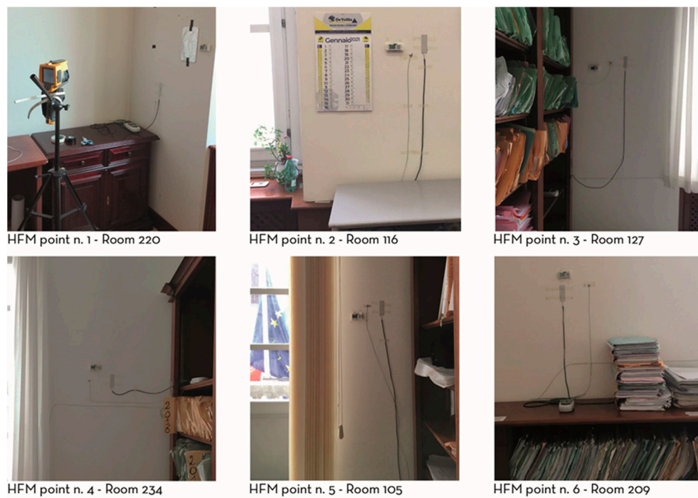
Figure 12. Example of installation of sensors for HFM measurements in 6 of the 9 rooms.
