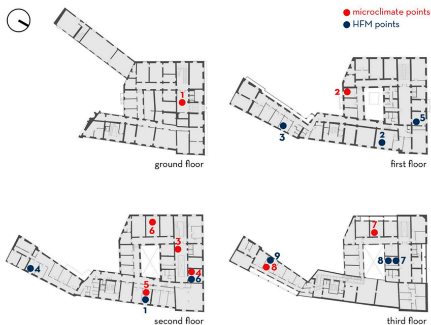
Figure 11. Locations and sensors code for indoor microclimate monitoring and HFM analysis divided by floor.
