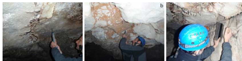
Figure 7. Surveying the carbonate rock mass and the breccia deposits in the Rondinella Cave by means of Schmidt hammer (a and b) and Barton profilometer (c).
