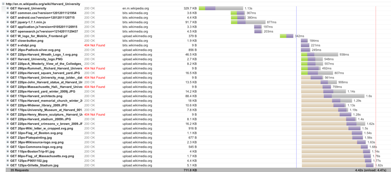
Figure 5. HTTP archive (HAR) capturing for Wikipedia: green is the connect time, purple is the wait time, and gray is the receive time.
