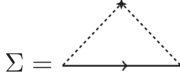
FIG. 1. Diagrammatic representation of the impurity self-energy in the self-consistent Born approximation. The solid line denotes the renormalized electronic Green's function, whereas the dashed lines connected by a cross represent the impurity scattering governed by the statistical correlations in Eq. (9).
