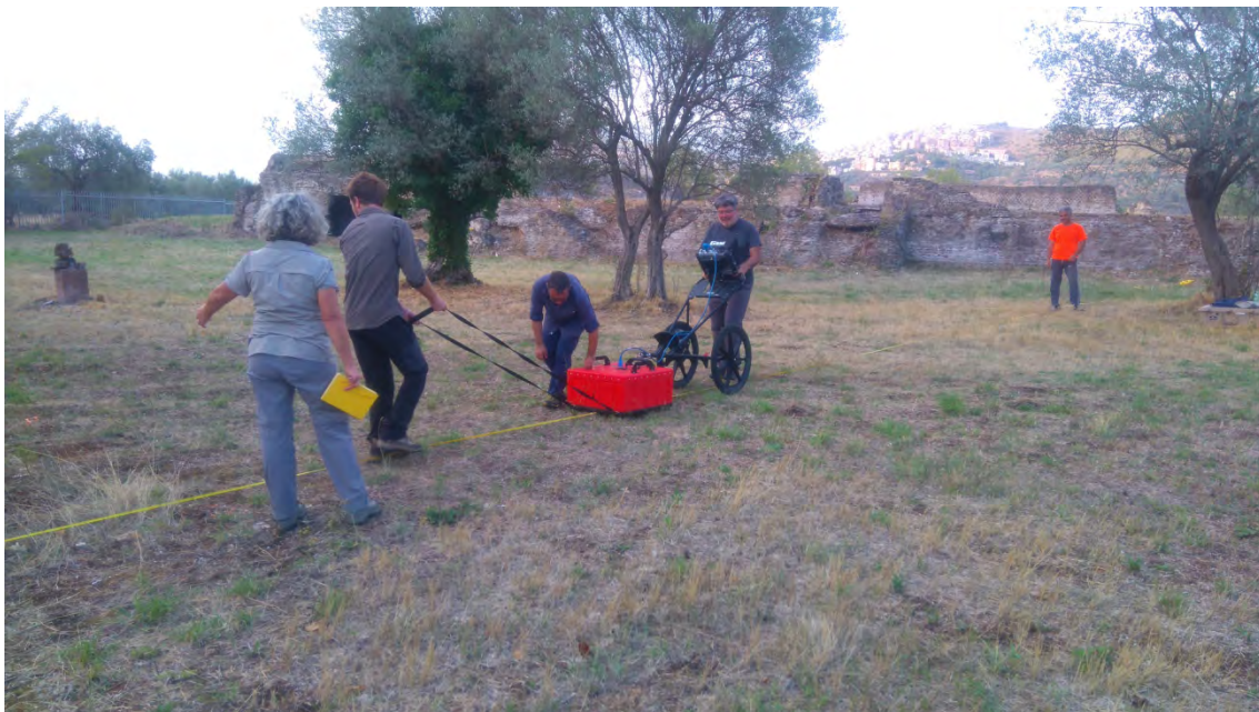
Figure 5. GPR system used to investigate the area and arrangement of operators.
