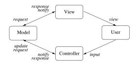
Figure 1: The MVC architecture and its communication protocol.
